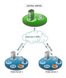
In OpManager, the site-level performance reports and network events can be extracted from both the central and probe web-clients. Further the user access can also be set at the remote-site probe and at the central server. This helps the remote admins navigate the desired information for the site they are in-charge of without affecting the centralized visibility.
